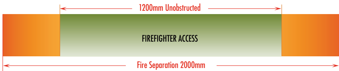
Figure 5 – Firefighter access and fire separation
