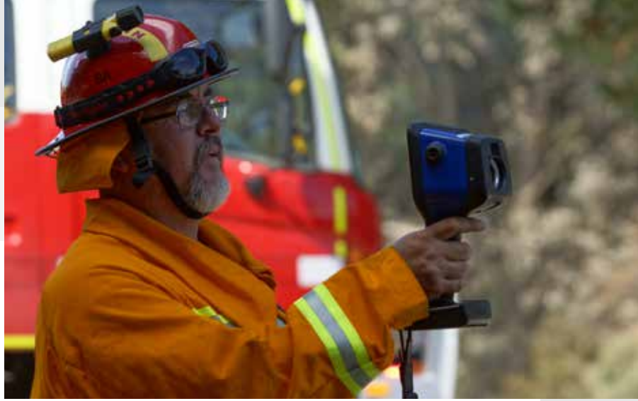
Used to detect heat sources, a thermal imaging camera is one of the most popular items chosen by brigades through the District Pick List Program.
