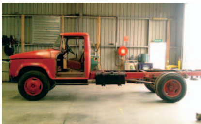
Tray and tank removed for sand blasting
